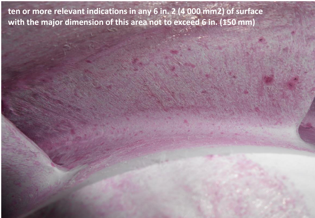
Photo 3: Detailed view of indications - after 60 minutes
